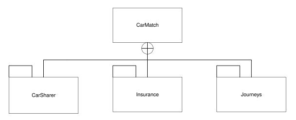
Tree Structured contained notation for packages in the CarMatch system
